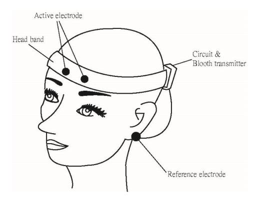
$Fig.\ 3.\ Illustration\ of\ the\ band-type\ EEG\ sensor\ attached\ to\ the\ head\ of\ a\ participant.$
