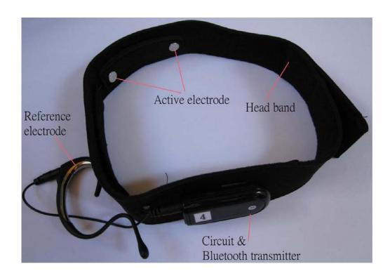
Fig. 2. The photo of the band-type EEG sensor.
